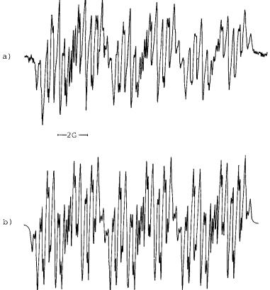
Figure 1. ESR spectrum of radical II: (a) observed; (b) simulated with a line-width of 0.21G.
